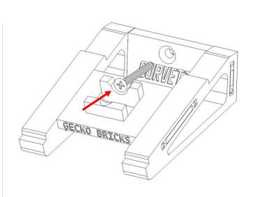
Install both screws into the back stretcher. Do not over tighten (use a screwdriver).
