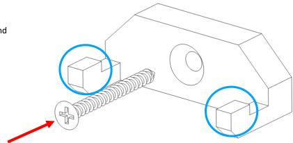
Do not over tighten (use a screwdriver).
