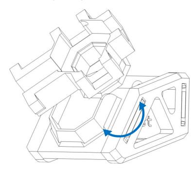
You can rotate the set to 8 positions and slide into the mount
