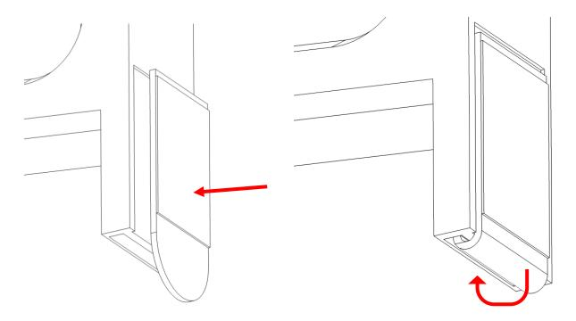
Use the included 3M command strip to prevent the mount from rotating around the fixing.
