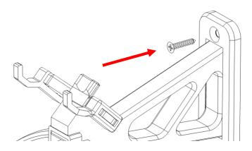
Use a Philips screwdriver to screw in the fixing. Do not over tighten.
